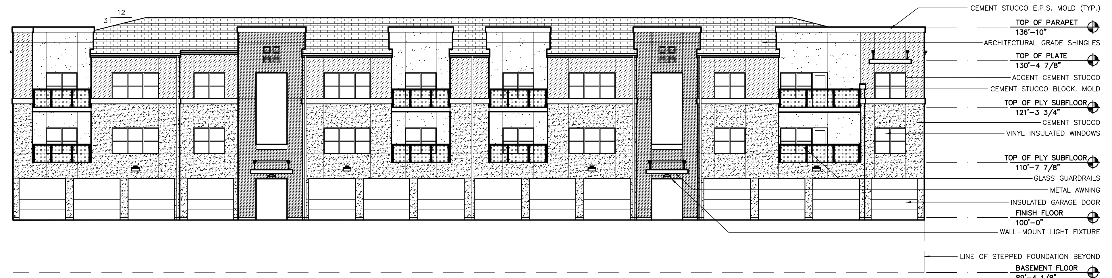
BUILDING TYPE 1 - FRONT ELEVATION SCALE: 3/32"=1'-0"
