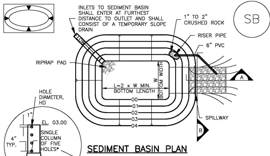
\*EXCEPT WHERE THE HOLES EXCEED 1" DIAMETER, THEN UP TO TWO COLUMNS OF SAME SIZED HOLES MAY BE USED
