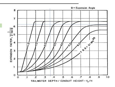
Figure 9-36. Expansion factor for rectangular conduits
