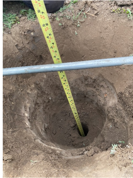
Photo 8 – Community 4's sandy loam and sandy clay loam soils didn't exhibit hydric soil indicators, and saturation and a water table were not encountered despite the soil pit extending to a depth of 38 inches.
