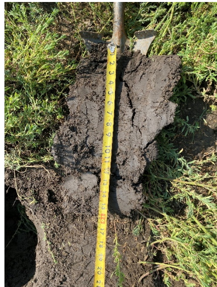
Photo 16 – Community 8's clay loam and silty loam soils didn't exhibit hydric soil indicators, and saturation and a water table were not encountered despite the soil pit extending to a depth of 48 inches.
