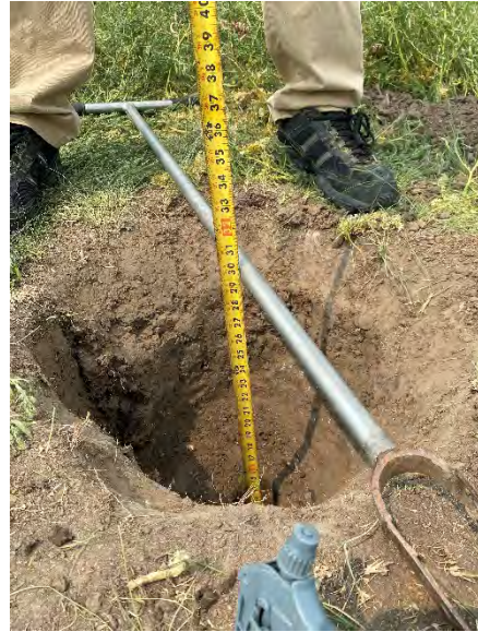
Photo 14 – Community 7's silty clay loam and sandy loam soils didn't exhibit hydric soil indicators, and saturation and a water table were not encountered despite the soil pit extending to a depth of 30 inches.
