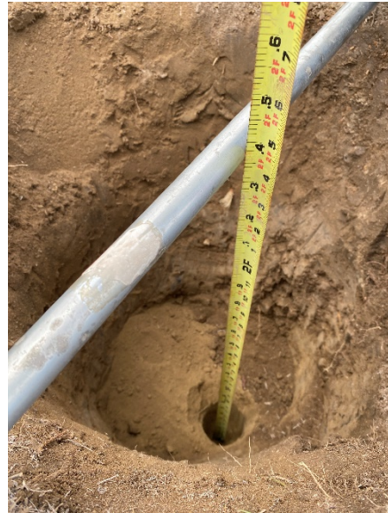
Photo 2 – Community 1’s sandy clay soils didn’t exhibit hydric soil indicators. Additionally, saturation and a water table were not encountered despite the soil pit extending to a depth of 28 inches.
