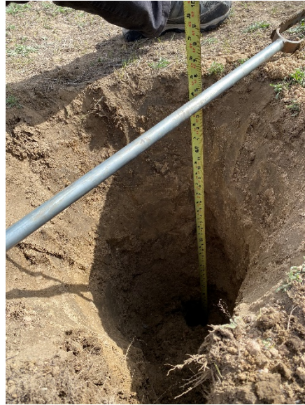
Photo 6 – Community 3's sandy loam, loamy sand and sand soils didn't exhibit hydric soil indicators, and saturation and a water table were not encountered despite the soil pit extending to a depth of 52 inches.
