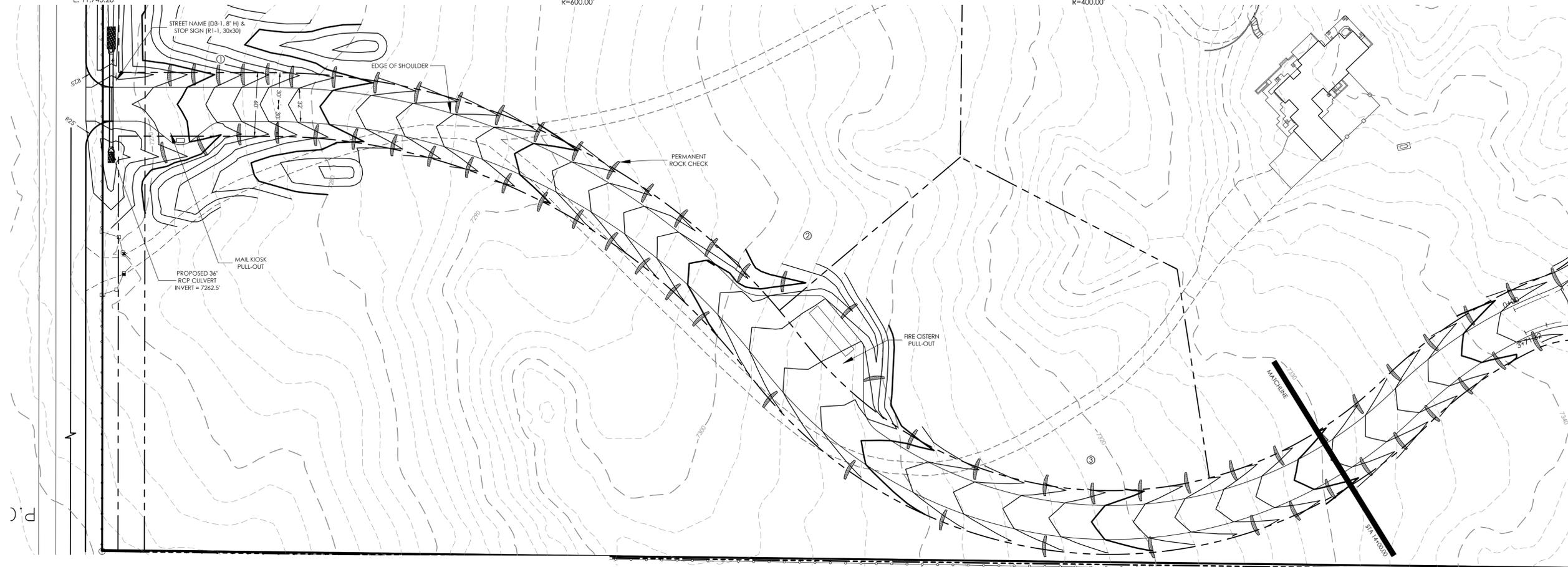
Please show ditch flowlines on profiles. Note that per ECM 2.5.8.C, ditches should have a minimum of 24 inch depth to accommodate driveway culverts.
