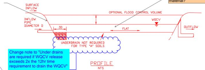
Change note to "Under drains are required if WQCV release exceeds 2x the 12hr time requirement to drain the WQCV"
