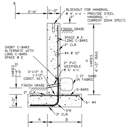
NOTE: WALLS ARE LESS THAN 4' HIGH AND ARE NON-ENGINEERED WALLS AND MAY VARY FROM THE DETAILS SHOWN
