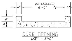
CURB IS IN A CATCH CONDITION UNLESS SPECIFIED AS SPILL
