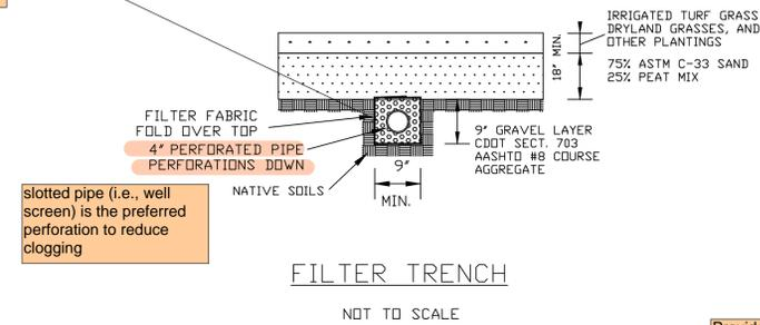
slotted pipe (i.e., well screen) is the preferred perforation to reduce clogging
