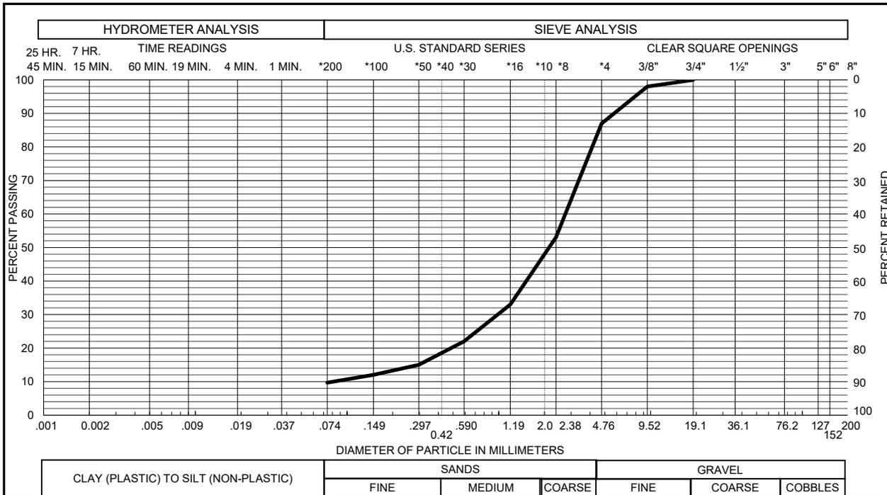
Sample of SAND, SLIGHTLY SILTY (SP-SM) GRAVEL 13 % SAND 77 %
