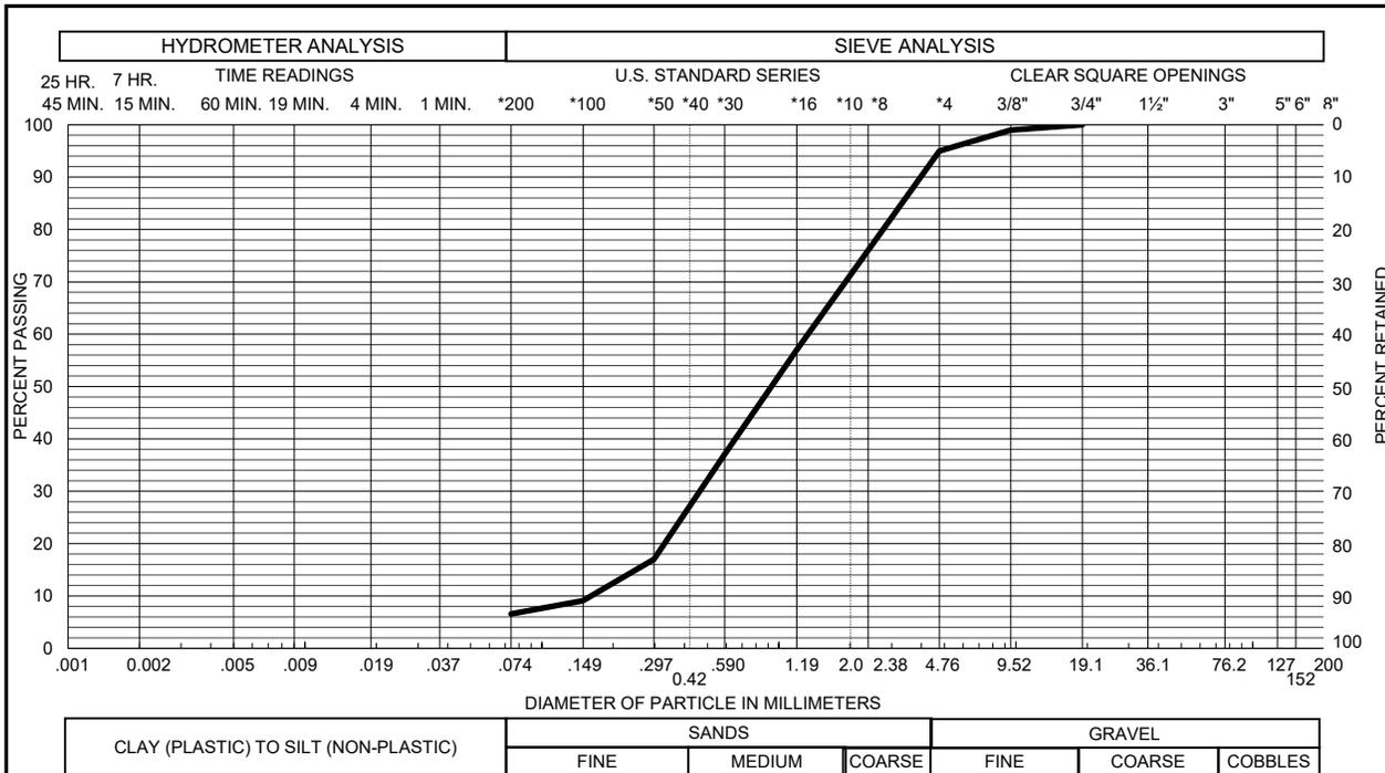
Sample of **SAND, SLIGHTLY SILTY (SP-SM)**      GRAVEL 5 %      SAND 88 %
