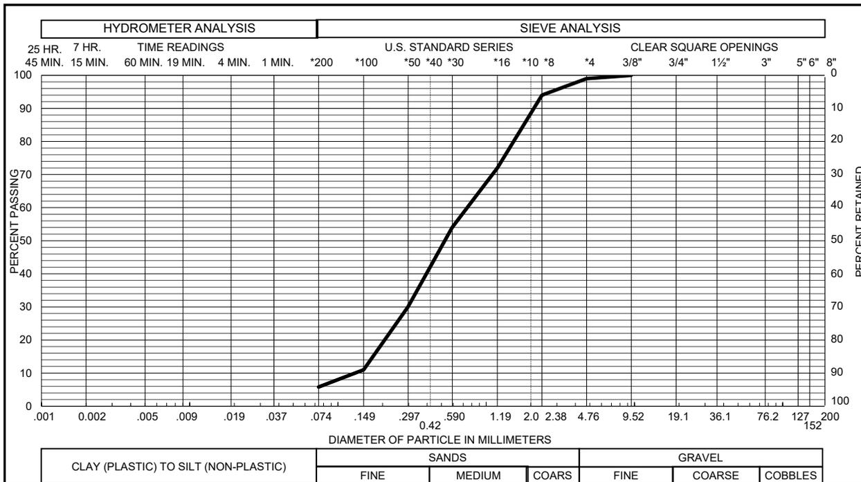
Sample of **SAND, SLIGHTLY SILTY (SP-SM)**      GRAVEL 1 %      SAND 93 %
