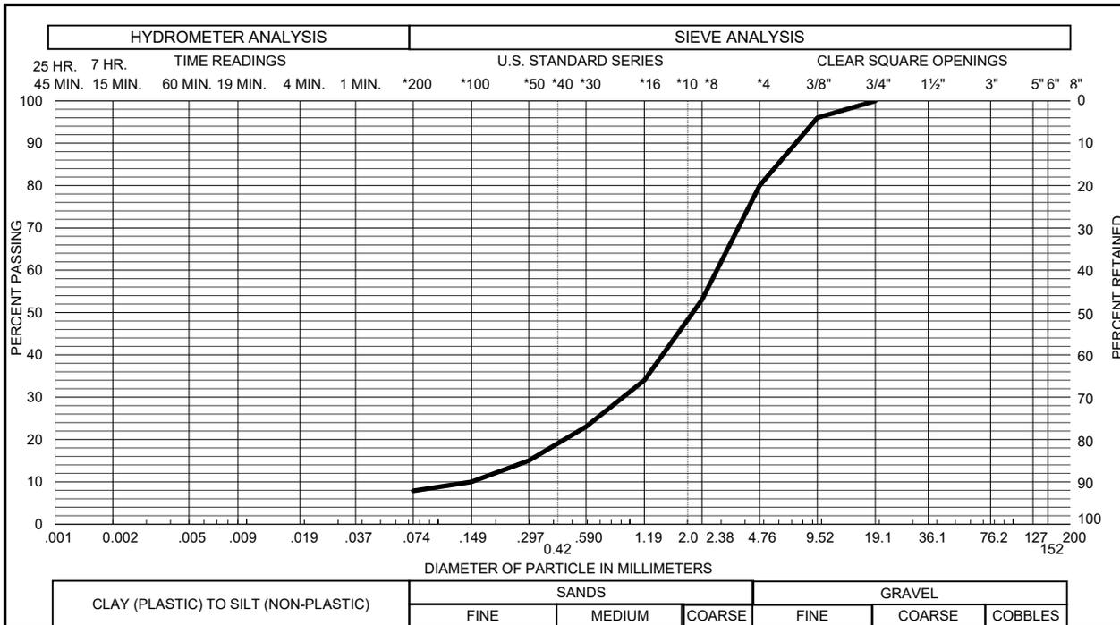
Sample of SAND, SLIGHTLY SILTY (SP-SM) GRAVEL 20 % SAND 72 %
