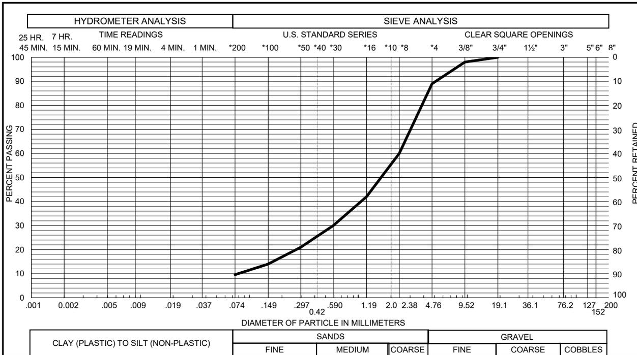
Sample of SAND, SLIGHTLY SILTY (SP-SM) GRAVEL 11 % SAND 79 %
