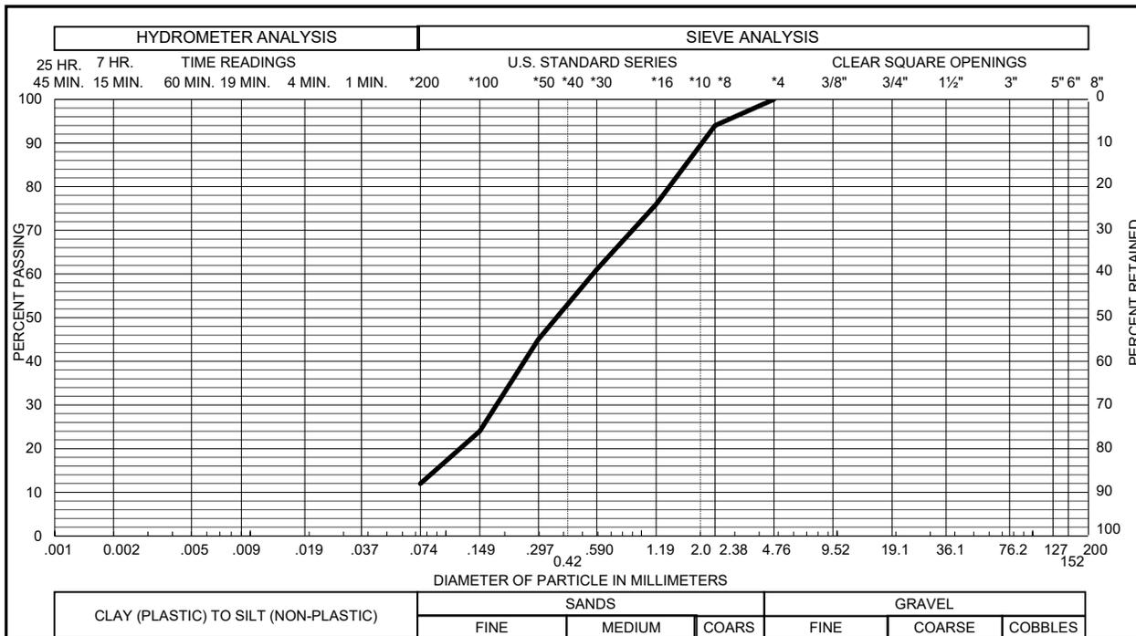
Sample of SAND, SLIGHTLY SILTY (SP-SM) GRAVEL 0 % SAND 88 %
