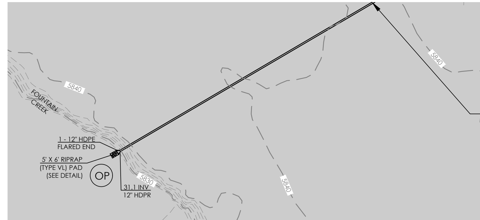
POND OUTLET PIPE DETAIL SCALE: 1" = 40'
