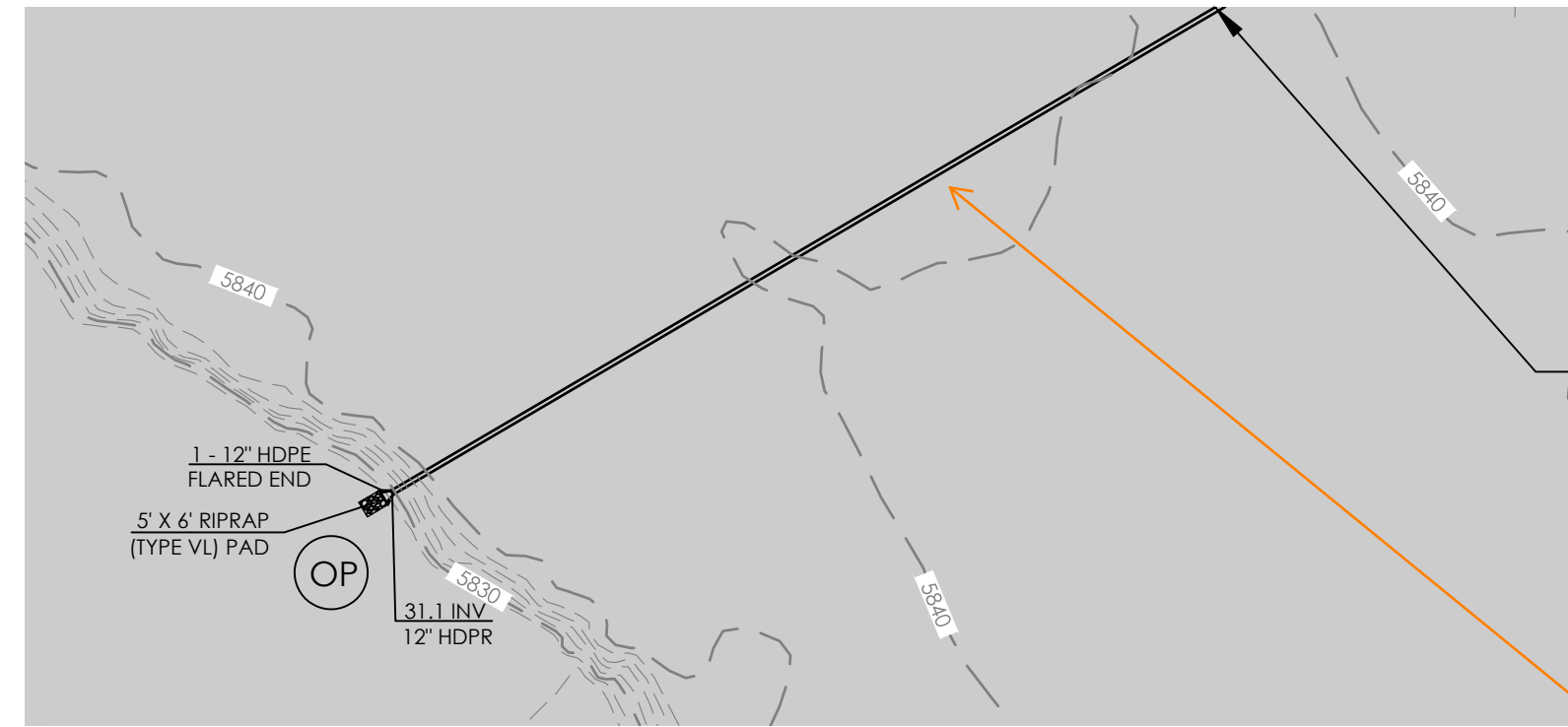
POND OUTLET PIPE DETAIL SCALE: 1" = 40'
