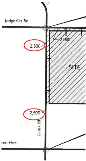
Existing ADTs on Curtis Road
