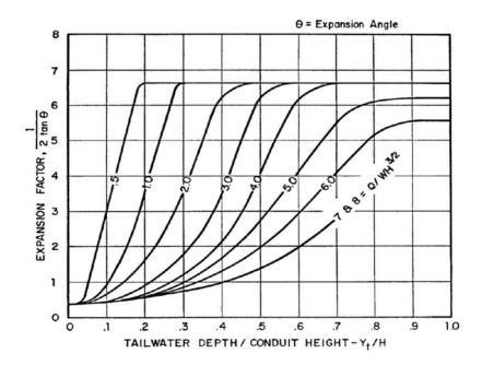
Figure 9-36. Expansion factor for rectangular conduits
