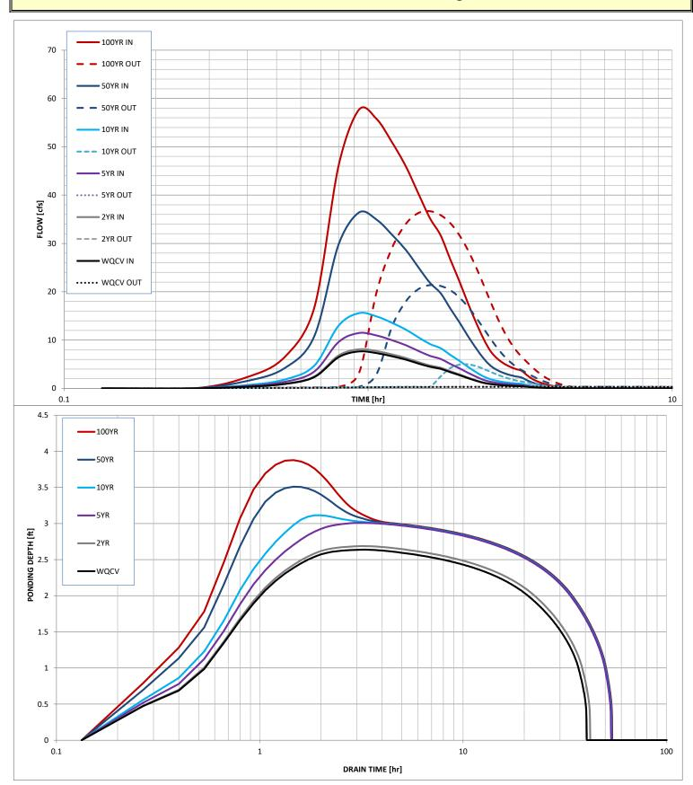
**Stormwater Detention and Infiltration Design Data Sheet**
