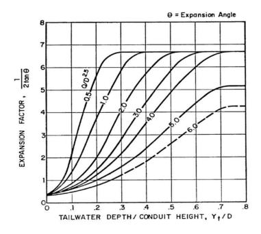
Figure 9-35. Expansion factor for circular conduits
