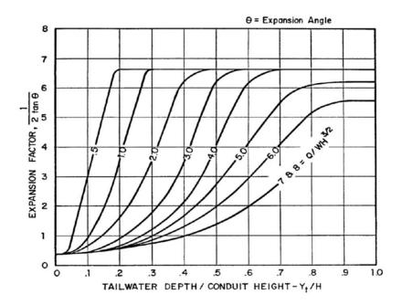
Figure 9-36. Expansion factor for rectangular conduits
