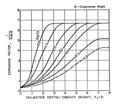
Figure 9-35. Expansion factor for circular conduits
