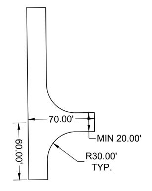
ACCEPTABLE ALTERNATIVE TO 120' HAMMERHEAD PER FALCON FIRE DISTRICT IFC CODE AMENDMENTS SECTION D103.1
