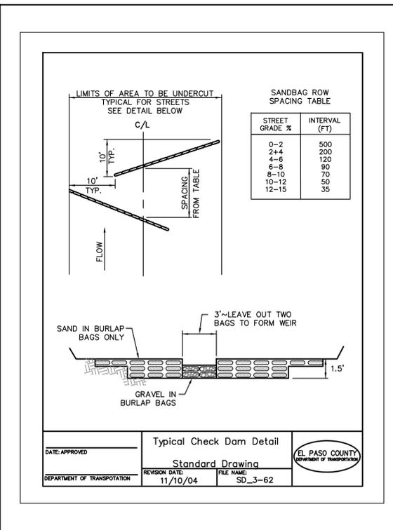
Typical Check Dam Detail Standard Drawing
