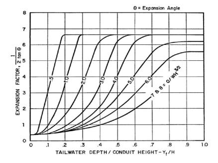
Figure 9-36. Expansion factor for rectangular conduits
