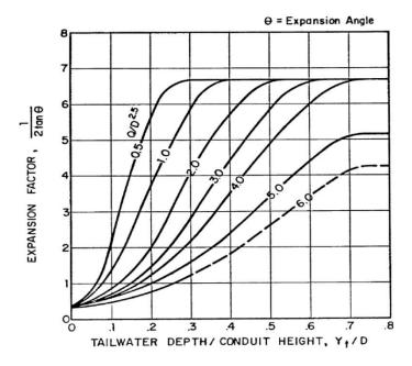
Figure 9-35. Expansion factor for circular conduits
