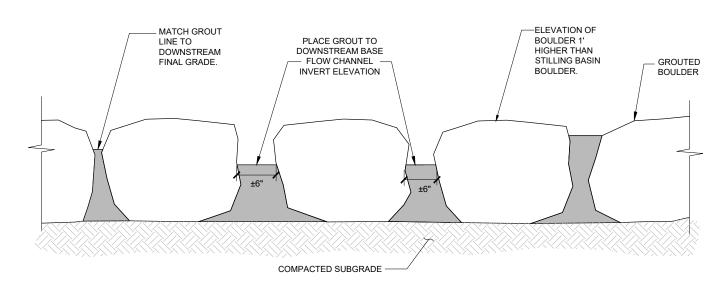
NOTE: ALONG THE END SILL, CORRESPONDING TO THE BASE FLOW CHANNEL, WIDEN GAP BETWEEN BOULDERS TO 6" AND MATCH TOP OF GROUT TO DOWNSTREAM INVERT AND STILLING BASIN INVERT (STILLING BASIN SHOULD BE FREE DRAINING).
