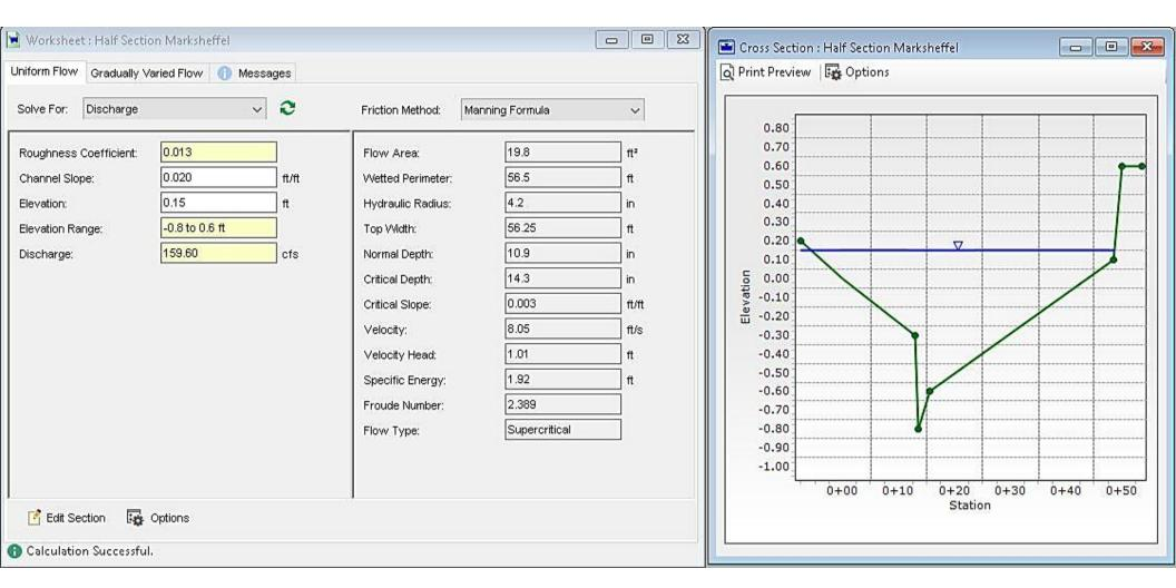
IF AN EMERGENCY OVERFLOW SITUATION WERE TO OCCUR, UPSTREAM BASIN'S (A6A, A7, A8, A9 A11, A15, A16, AND A21) 100 YEAR RUNOFF WOULD TRAVEL DOWN MARKSHEFFEL ROAD AND SHEET FLOW INTO SAND CREEK. THE TOTAL 100 YEAR RUNOFF OF THESE BASINS IS 126.7 CFS.
