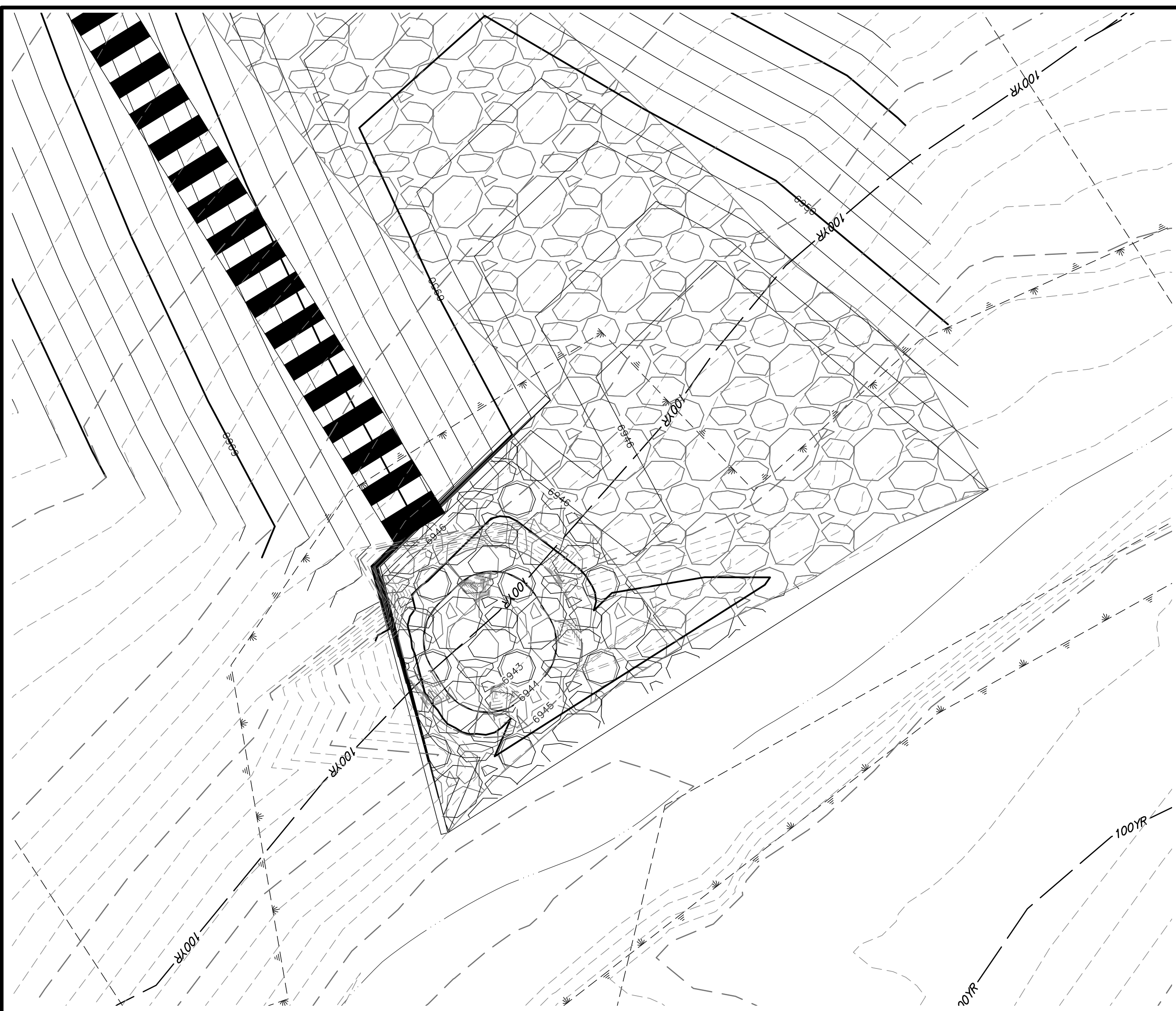
STORM 23 - 84" OUTFALL STILLING BASIN W/ HEADWALL & WINDWALL
