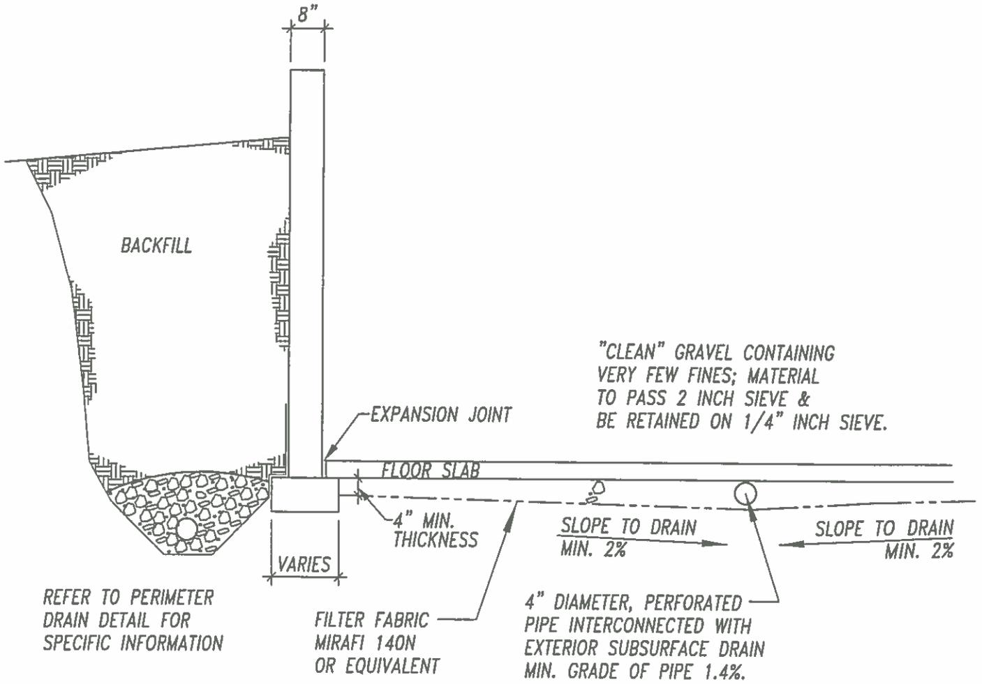
4.11e Detail Room\Drawings\UNDERSLAB CAPILLARY BREAK DRAIN Area Layout.dwg 6/12/2007 12:11:50 PM
