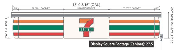
**ELECTRICAL NOTE**: EXPOSED EXTERIOR 20 AMP WEATHERPROOF ELECTRICAL DISCONNECT REQUIRED WITHIN VISUAL RANGE OF SIGN REQUIRED FOR EVERY 16 AMPS OF SIGNAGE. ACTUAL NUMBER OF CIRCUITS TO BE DETERMINED BY A LICENSED ELECTRICAL CONTRACTOR. ACTUAL LOCATION OF BOX MAY VARY. CIRCUITS AND SWITCH TO BE PROVIDED BY OTHERS. INPUT VOLTAGE - 120V ALL SIGNAGE WILL BE (MET) LISTED, (U.L.) 48STD COMPLIANT AND CARRY (MET) LABELS.
