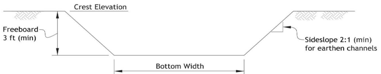
Spillway Section
