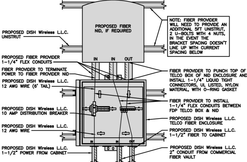
LIT TELCO BOX – INTERIOR WIRING LAYOUT (OPTIONAL)
