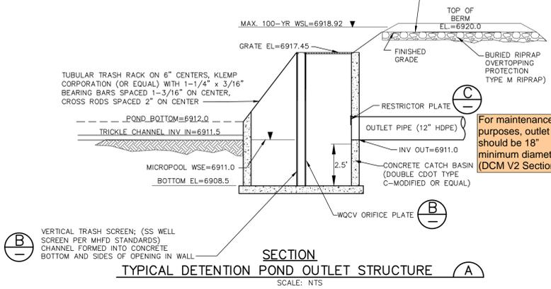
VERTICAL TRASH SCREEN: (SS WELL SCREEN PER MHFD STANDARDS) CHANNEL FORMED INTO CONCRETE BOTTOM AND SIDES OF OPENING IN WALL
