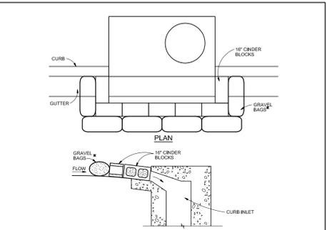
**BLOCK AND GRAVEL BAG CURB INLET PROTECTION**
