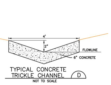
Pond bottom should have a minimum slope of 3% to the trickle channel
