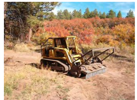
Figure 4. Mechanical treatment using a timberaxe.
