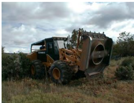
Figure 3. Mechanical treatment using a Hydroaxe®.
