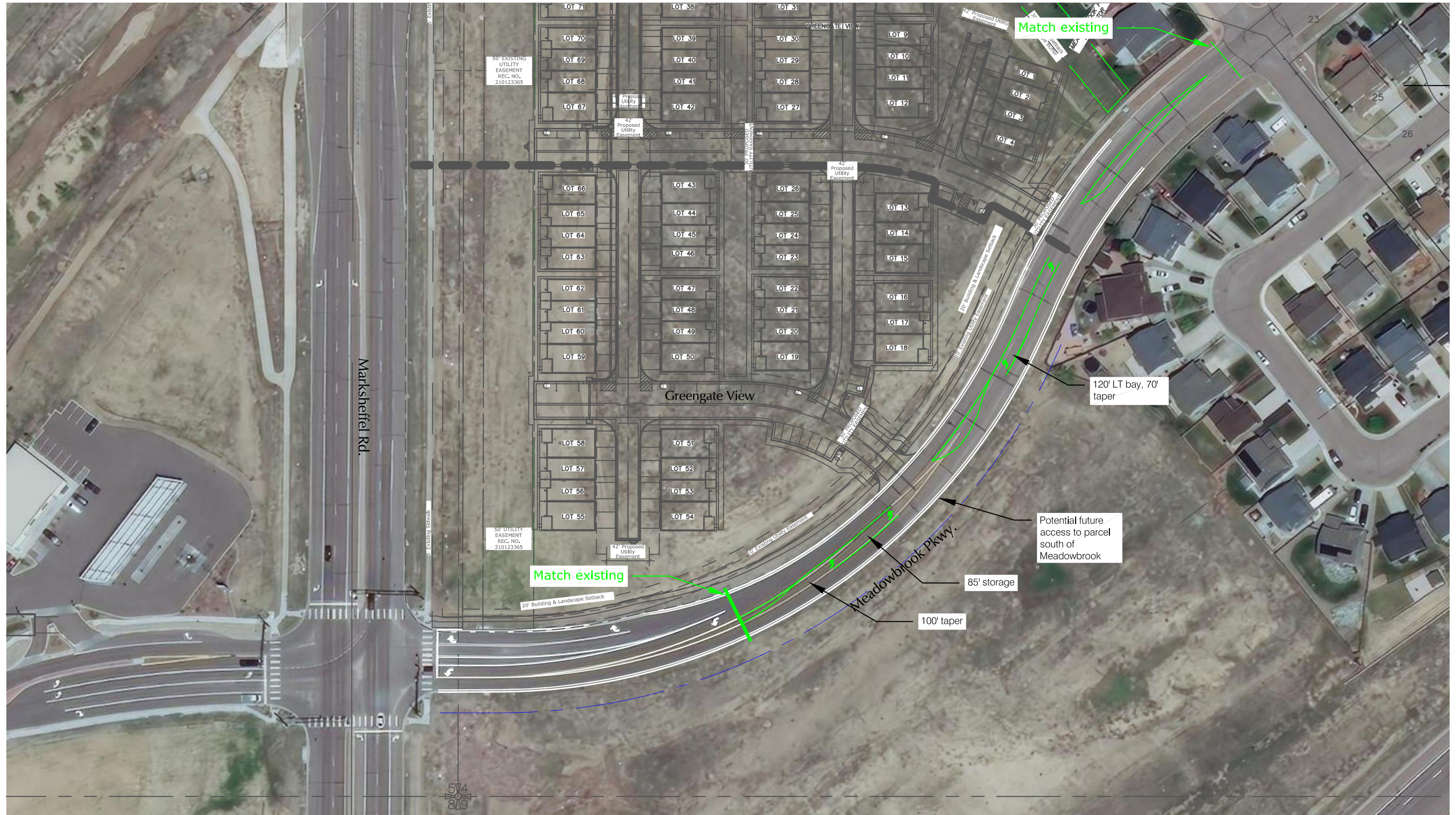
Figure 10 Conceptual Restriping Plan Meadowbrook Parkway Villas at Claremont Ranch (LSC #204130)
