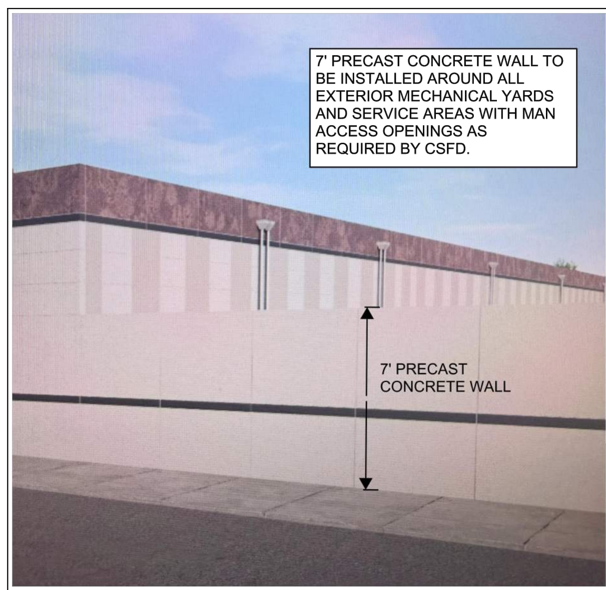
PRECAST CONCRETE WALL DETAIL (NOT TO SCALE)
