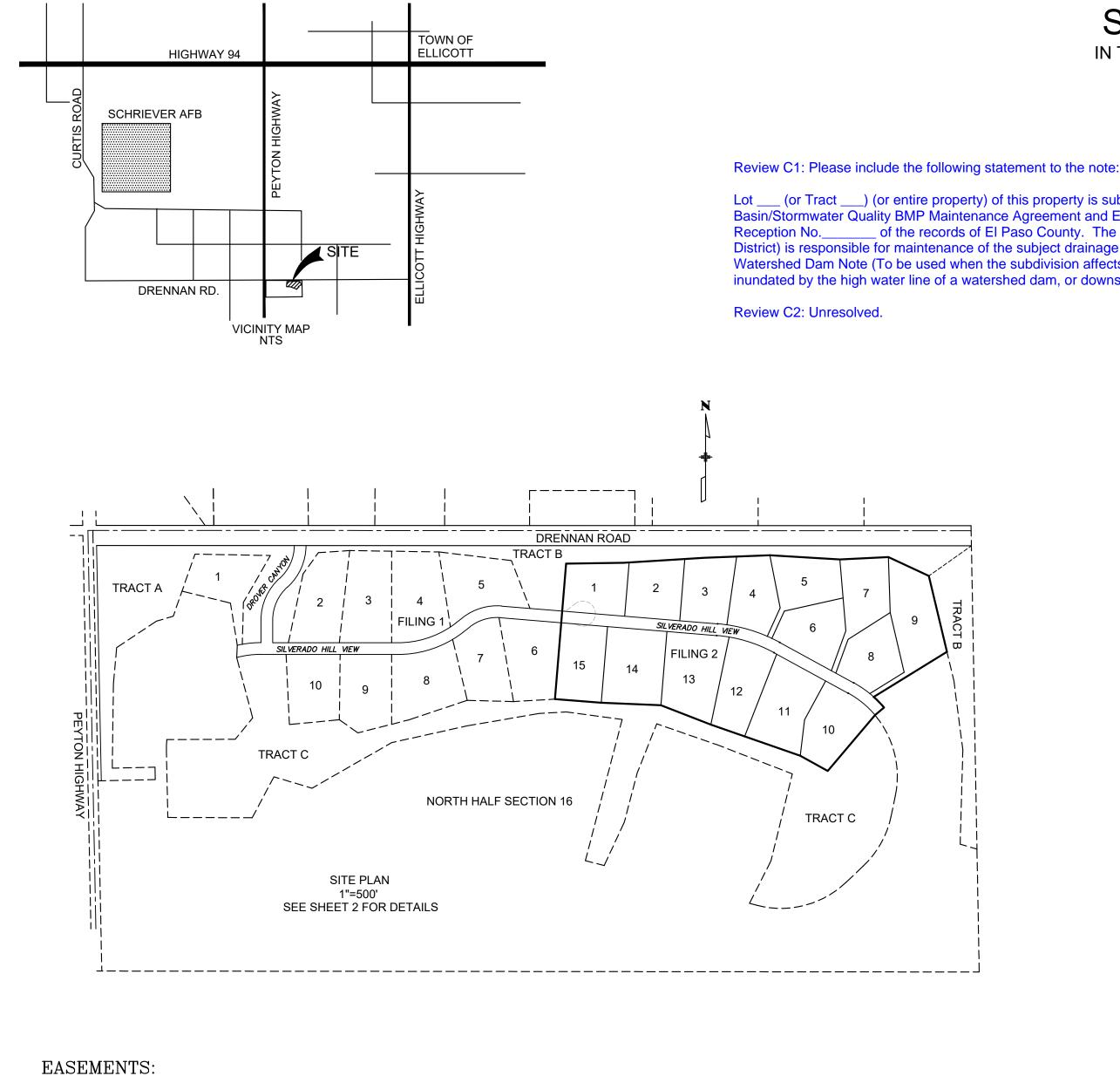
SIDE, FRONT AND REAR LOT LINES ARE HEREBY PLATTED WITH A TEN (10) FOOT EASEMENT FOR DRAINAGE AND PUBLIC UTILITIES ONLY, WITH THE SOLE RESPONSIBILITY FOR MAINTENANCE BEING VESTED WITH THE PROPERTY OWNERS.
