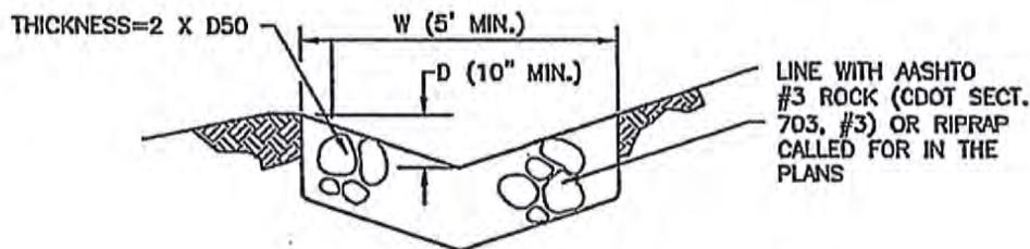
DS-5. RIPRAP LINED SWALEEARTH DIKE AND DRAINAGE SWALE INSTALLATION NOTES
