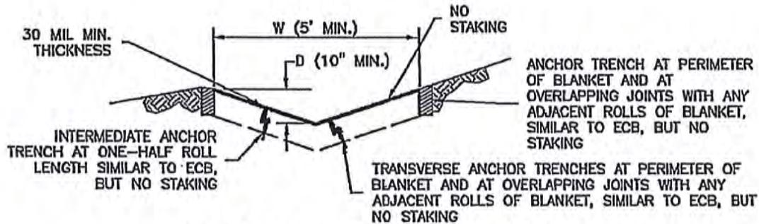
DS-4. SYNTHETIC LINED SWALE
