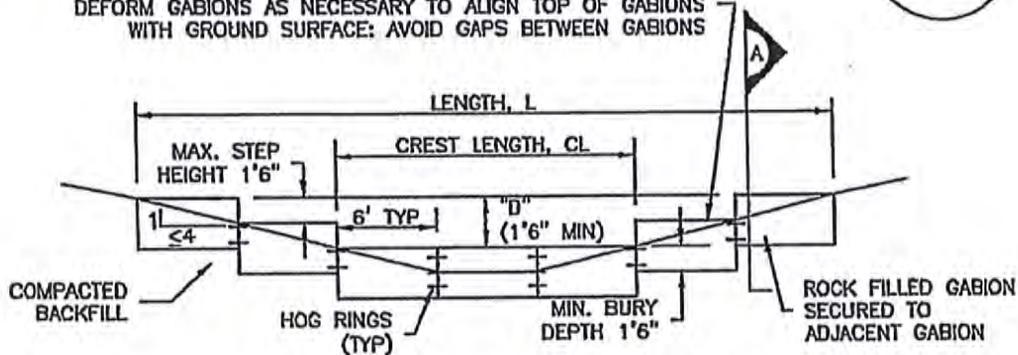
REINFORCED CHECK DAM ELEVATION VIEW
