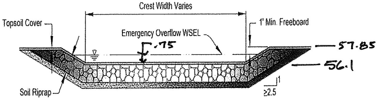
Figure 13-12d. Riprap Types for Emergency Spillway Protection
