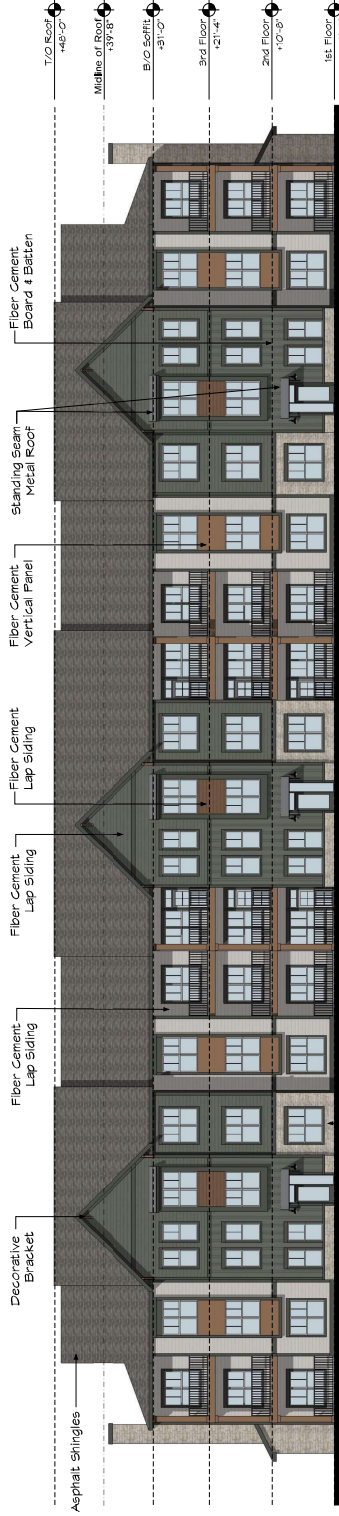
FRONT ELEVATION - BUILDING TYPE B Scale: 3/32" = 1'-0"
