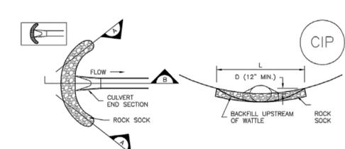
CIP-1. CULVERT INLET PROTECTION
