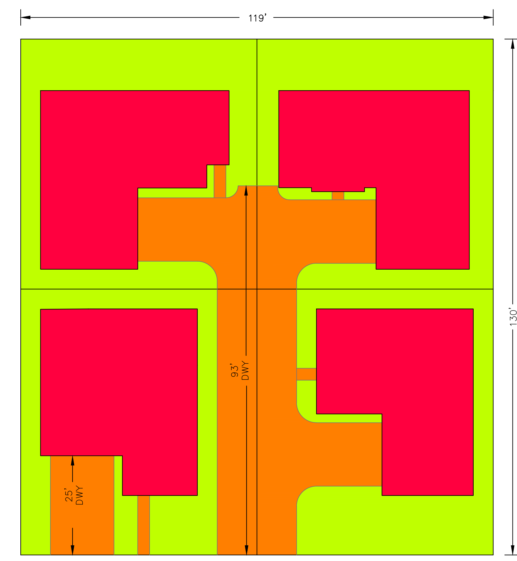
TYPICAL HOME LOT UA = 42% OF LOT AREA DCIA = 22% OF LOT AREA RPA = 36% OF LOT AREA
