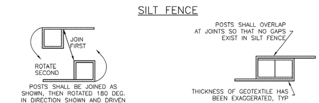
SF-1. SILT FENCE
