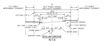
The 'Modified Private Road Cross Sections' reduced the pavement widths to allow minimum 10-foot travel lanes of the typical local urban low volume cross section of the private roads equivalent travel surface/lanes width same pavement width as. As depicted on the PUD and associated private road cross sections and details, adequate provision has been made for water/wastewater utility lines within the private road easement.
