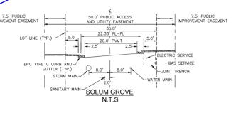
The 'Modified Private Road Cross Sections' reduced the pavement widths to allow minimum 10-foot travel lanes of the typical local urban low volume cross section of the private roads equivalent travel surface/lanes width same pavement width as. As depicted on the PUD and associated private road cross sections and details, adequate provision has been made for water/wastewater utility lines within the private road easement.
