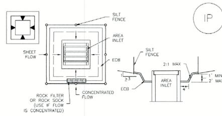
**IP-5. OVEREXCAVATION INLET PROTECTION**
