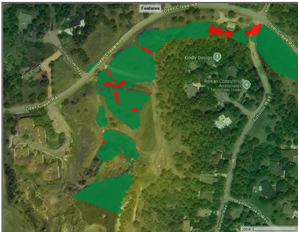
Figure 4. High Shear Stress Areas (Froude Number \geq 0.9 )
