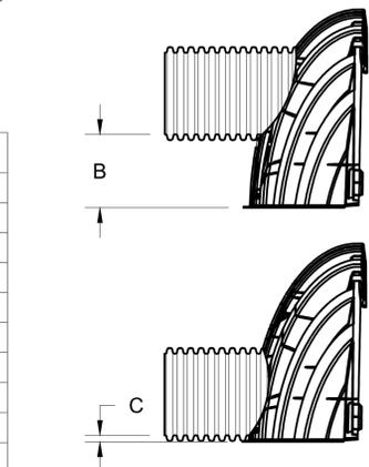
CUSTOM PREFABRICATED INVERTS ARE AVAILABLE UPON REQUEST. INVENTORIED MANIFOLDS INCLUDE 12-24" (300-600 mm) SIZE ON SIZE AND 15-48" (375-1200 mm) ECCENTRIC MANIFOLDS. CUSTOM INVERT LOCATIONS ON THE MC-7200 END CAP CUT IN THE FIELD ARE NOT RECOMMENDED FOR PIPE SIZES GREATER THAN 10" (250 mm). THE INVERT LOCATION IN COLUMN 'B' ARE THE HIGHEST POSSIBLE FOR THE PIPE SIZE.
