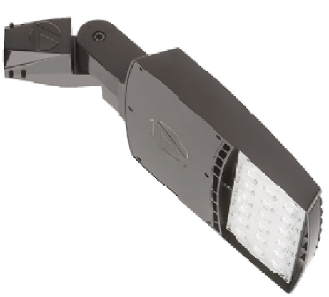
TYPE F1 LITHONIA RSKXF1 LED WIDE FLOOD CUT-OFF VISOR TO LIMIT SPILL LIGHT 10,600 LUMENS, 4000K POLE MTD TO ILLUMINATE BEACH AREA
