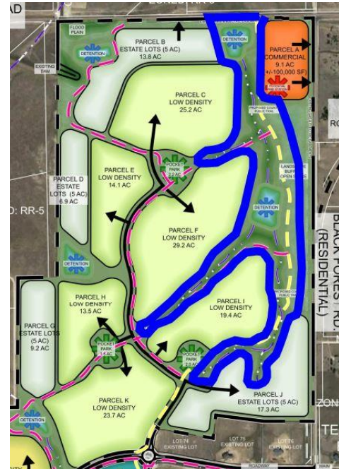
Figure 16--Existing drainage ways are preserved within open space corridors (blue highlighted area).
