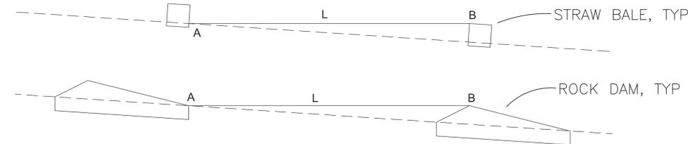
L= THE DISTANCE SUCH THAT POINTS A AND B ARE AT THE SAME ELEVATION.
