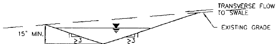
DS-1. COMPACTED UNLINED EXCAVATED SWALE
