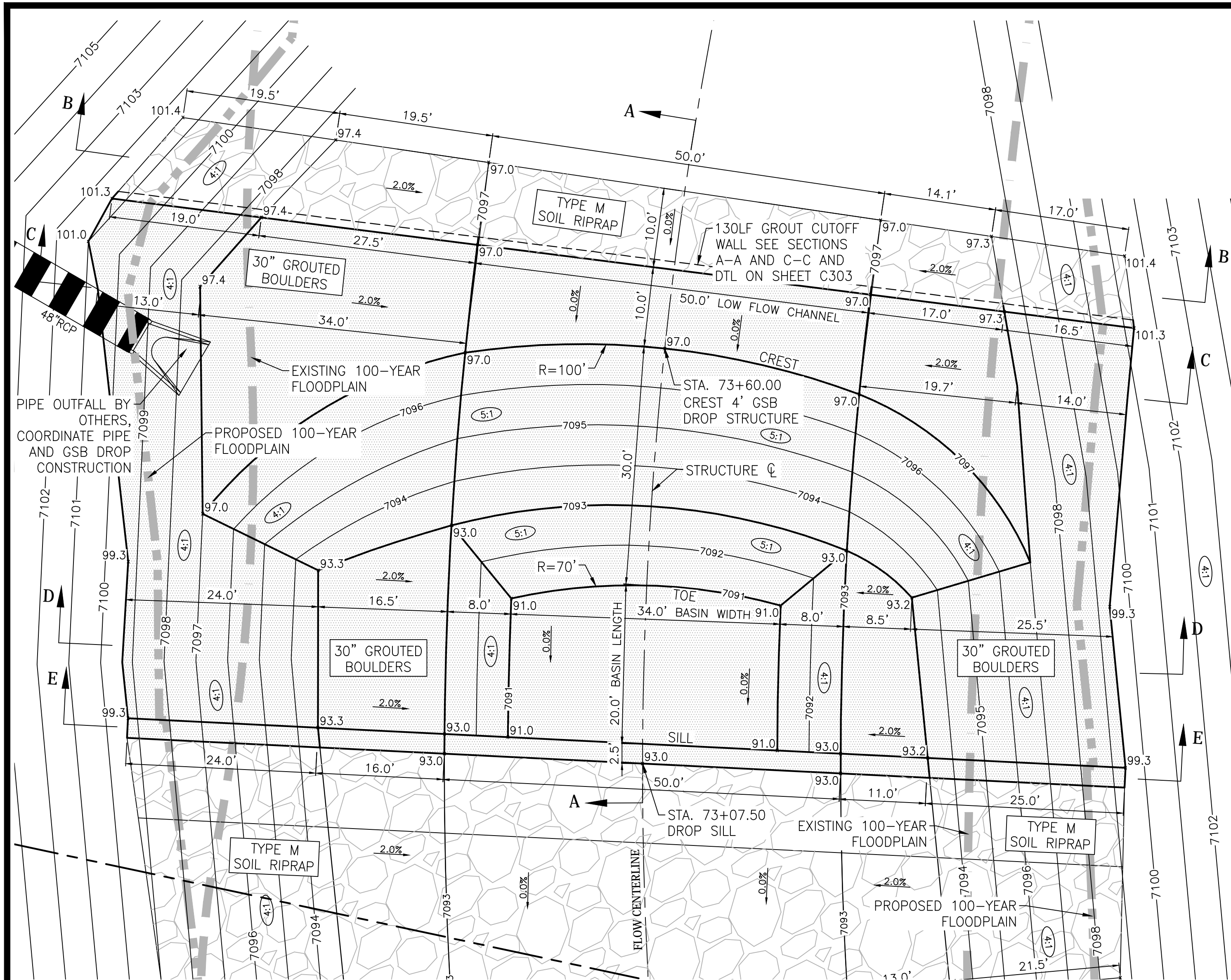
DROP STRUCTURE A PLAN 1"= 10'
