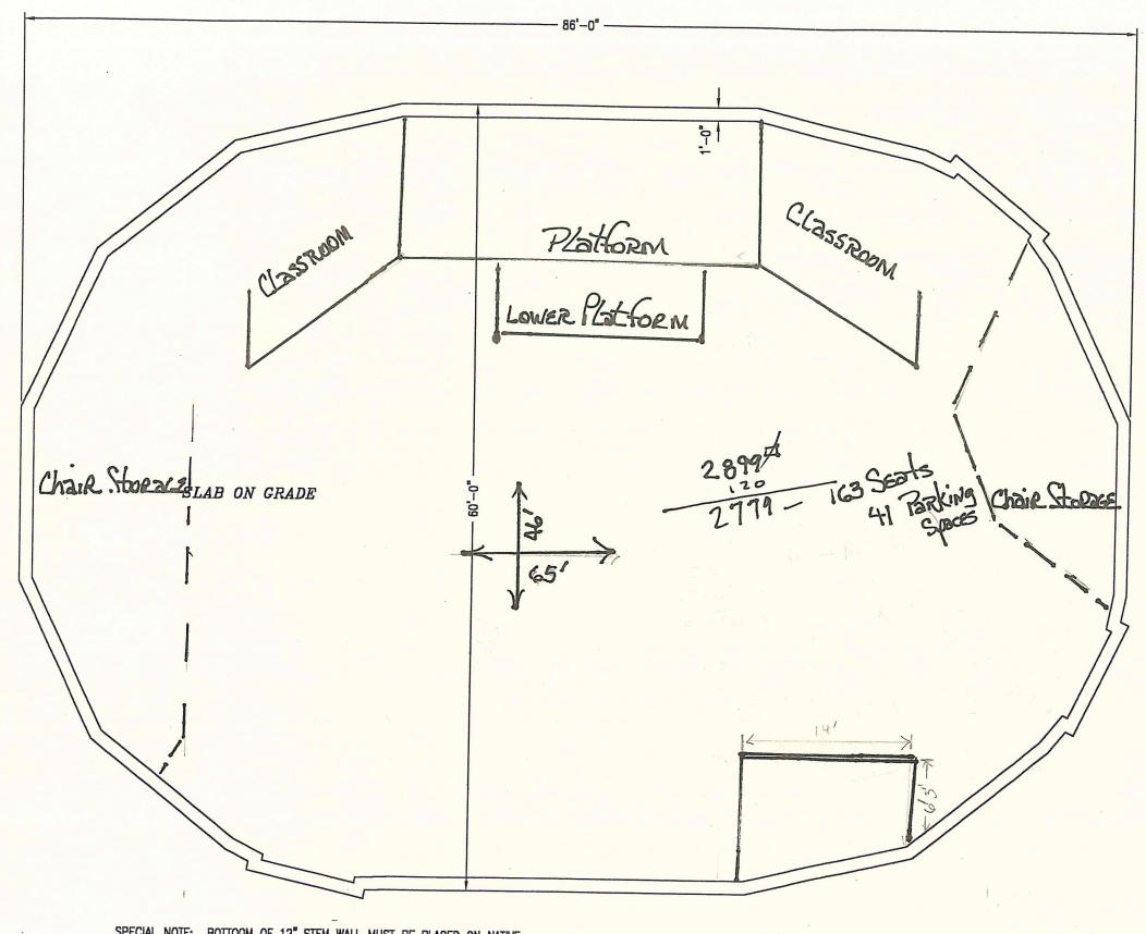
SPECIAL NOTE: BOTTOOM OF 12" STEM WALL MUST BE PLACED ON NATIVE SOIL. THERE IS SOME FILL MATERIAL ON SITE AND THE WALL MUST PENETRATE ANY FILL MATERIAL. IT IS OPTIONAL TO REPLACE FILL MATERIAL WITH COMPACTED STRUCTURAL MATERIAL.
