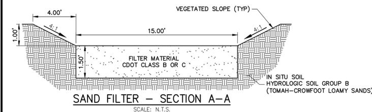
SAND FILTER - SECTION A-A
