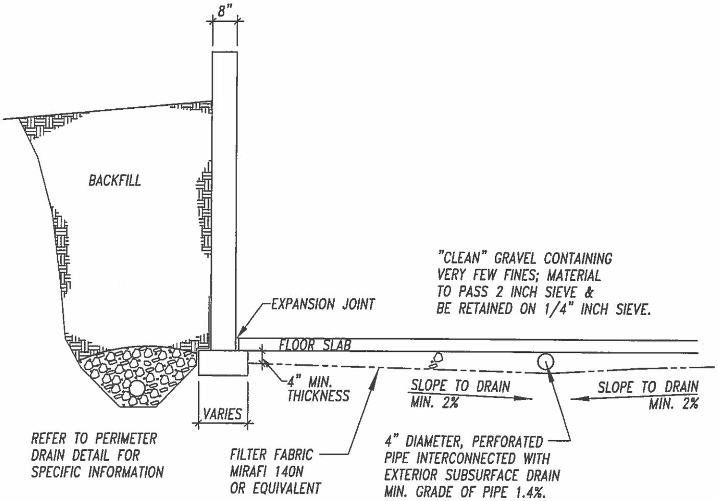
411e Detail RevA Underslab Drainage Capillary Break Drain.dwg, L:\work\1\_6\112007\12-11-06 PM 1:48
