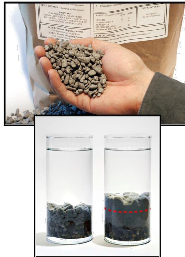
Figure 1. Configuration of stone-clay composite particle.
