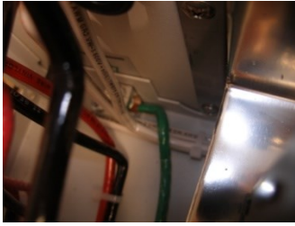
Chassis ground connection to inverter
