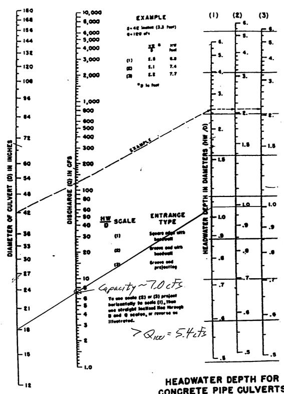
HEADWATER SCALES 283 NEVISED MAY 1964 CONCRETE PIPE CULVERTS WITH INLET CONTROL
